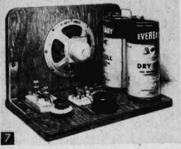
This buzzer "amplifier" is ideal for use wherever a large number of persons assemble to learn the code. No vacuum tubes are used, yet speaker volume is more than enough to fill a large hall.
