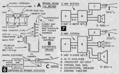
Fig. 6. Comparison of (A) moving coil loud speaker (B) electrostatic speaker (C) Ionovac, shows the much greater simplicity of the ion-cell's sound reproducing structure. Connecting to hi-fi layouts (Fig. 7) would not be difficult.
