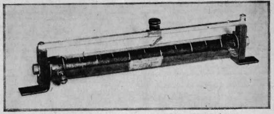
The finished slide wire resistor. This one has a value of 5000 ohms, 200 watts, .2 amperes.
