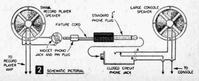
Record player and console speakers are operated in parallel by plug-in cable. Removal of plug from telephone jack automatically restores console speaker to normal operation.
