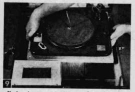
Placing changer, mounted on the motor board, down onto motor board support strips.
