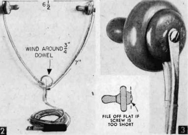
for the price you would ordinarily pay for a cheap pair of magnetic earphones! This crystal headset has much to recommend it. Its sensitivity, frequency range, and clarity of reproduction are superior to magnetic type earphones. Also, it weighs less than two ounces, is easy to assemble, and its  $6\frac{1}{2}$
