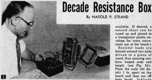
Decade resistance box in use in radio servicing job. Various values of resistance are being applied across terminals where a defective resistor was formerly soldered, and which is now unidentifiable due to extreme heating.
