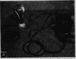
A 150-watt lamp is connected in series with motor to reduce its speed when test running.
