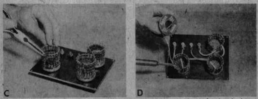
With the resistor equipped switches attached to the 'panel, attach formed rings of bare copper wire to free loops, bending them down uniformly over the ring (C); and after the three rings have been placed and leads connected as shown, solder all points of contact to the rings.
