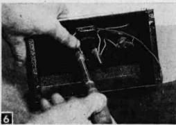
Wire connections inside the cabinet are very simple, with two resistors required as shown.
