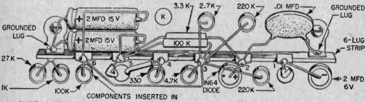
CLOSE-UP DETAILS OF TIE-STRIP CHASSIS HOLES LOOKING DOWN ON CHASSIS
