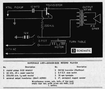
ume will not be disturbingly loud. But by changing the size of the 220K ohm resistor the volume and tone quality can be varied. Before experimenting with such a change, however, insert a 0 to 10 ma meter in series with the battery so that the transistor will not be damaged. The transistor should never pull over 5 ma; with the fixed value of resistance given in Fig. 3 and the Materials List, transistor current is slightly over 2 mills. Be sure to observe correct battery polarity.
