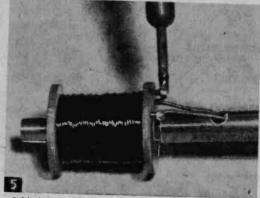
Soldering flexible leads to terminal pins, after movable magnet's core has been pressed into pendulum tubing. Avoid too much heat on pins or they may loosen in plastic.
