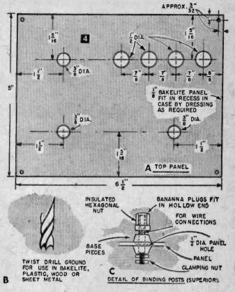
marked point and install, using a washer on each side of the panel, applying cement (such as coil dope) to the lower washer to keep the switch from turning and to keep the dial plate, top washer and nut clamp assembly tight. Then install knobs.
