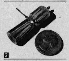
In this hi-fi addict's Sherlock Holmesian closeup nothing goes unnoticed. Small polat at top is one golden lonizing electrode lead. Small wire loop around quartz chamber's wasp waist is second ionizing electrode. Air cloud is ionized in long hollow end which narrows at waist to aperture the diameter of an automatic-pencil lead. Cloud is similar electrically to earth's ionosphere.
