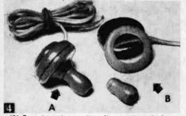
(A) Crystal earphone unit as it comes from dealer-(B) After front cover has been removed and opening enlarged with rat-tail file. Cover rim is then snapped back on, without injury to diaphragm.
