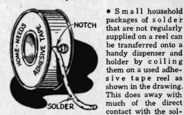
der and any escaped flux. Cut a hole at the side of the can for uncoiling the solder. A wedgeshaped notch at the side of the hole will lock the solder from receding back into the can.
