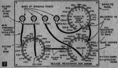
ing it to make sure that the marked value is accurate to within plus or minus 10% of its markings. When, as occasionally will happen, a resistor is found that is inaccurately marked. substitute another. (If 5% or 1% resistors are used, testing is not necessary. If you are unfamiliar with resistor color coding, an IRC Resist-O-Guide can be obtained for 15¢ from any electronics supply store,) With all resistors sol-
