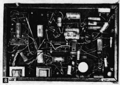
Under chassis view of 7-in. conversion. Scope was built on new chassis, using some new components, many from TV set converted (see Fig. 3).
