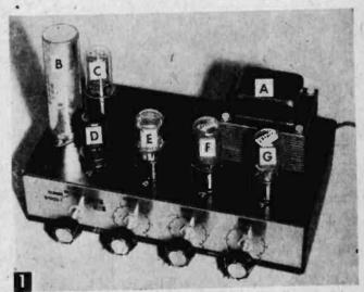
Completed amplifier. Controls, left to right, are: Selector Switch, Volume, Bass, and Treble (line switch) controls. Escutcheon plate may be removed from chassis and mounted on cabinet if unit is enclosed. Parts shown are: A) power transformer; B) electrolytic capacitor; C) 5Y3GT rectifier; D) 6SC7 dual pre-amplifier; E) 6SLF Interstage amplifier and phase inverter; F & G) 6V6 beam power push-pull output amplifiers.
