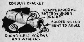
in front of battery so it contacts center electrode. Use one of conduit bracket mounting screws, and screw holding soldering lug, for binding screws across rear top edge to secure it.
