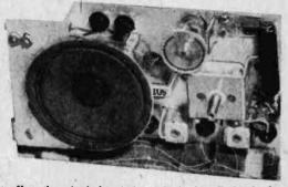
Here the wired chassis is ready for installation in the case. A flat ferrite core antenna is shown fitted in a plastic holder at the bottom.
