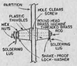
panel, cabinet or partition which will give ample clearance for brass screw or rod, to avoid shorts or losses, and assemble with thimbles and nuts as shown in drawing. Since heat will melt or soften the plastic thimbles, make solder connections to solder lugs before bolting onto thimbles.
