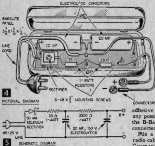
20 mf., 150 w.v. electrolytic capacitors were arranged so both negatives were to the center of the Bakelite strip. The pigtail leads were then laced through the  $\frac{1}{16}$  holes (Fig. 4) as shown in the pictorial. With all but  $\frac{1}{2}$  in. of each lead clipped off, the wires were formed into small loops with flatnose pliers. These loops made perfect soldering lugs for attaching resistors and flexible wire leads.
