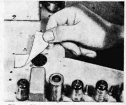
• When soldering on top side of radio or TV chassis, dropping solder in an open tube socket can cause trouble. Eliminate this possibility by placing a strip of wide adhesive tape over the open socket.—H. LEEPER.
