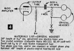
the connections to one earpiece to see when the reproduction sounds the most natural. A pair of phone cord tips or a midget phone plug soldered to the free ends of the cord will complete the headset.
