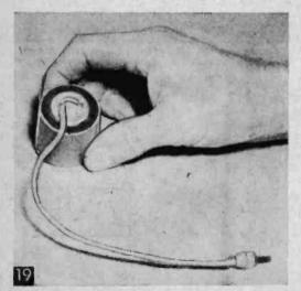
Microphone mounted in insulating rubber ring, which in turn is fitted into Bakelite tubing mouthpiece.
