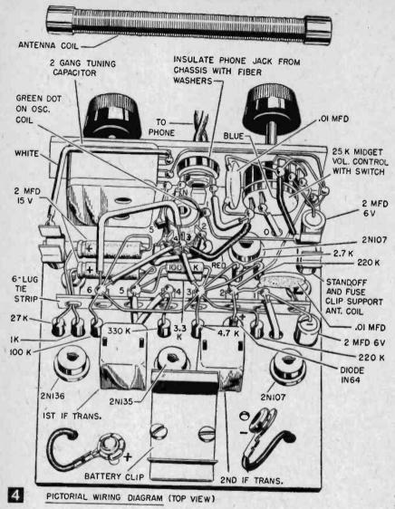
The set's pee-wee dimensions are made possible through use of a sub-miniature two-gang, plastic encased tuning capacitor, volume control, phone jack, and I.F. transformers. These parts are readily available from the source given in the Materials List. When completed, this tubeless transistorized superhet will be no larger in size than two packages of king-size cigarettes.
