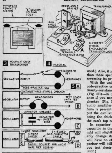
MATERIALS LIST-SCOTSMAN'S DELIGHT No. Rea'd Description 1 3/4x4x4" pine or plywood DC #6x1/2" r.h. wood screws brass angle bracket, 11/2'' arms iron angle bracket, 11/2'' arms 1 1 2 Fahnestock clips CK722 Raytheon transistor 1 Thordarson 20-A-16 transformer (or Stancor A-53 or Triad A-31X) 22,000 ohm, 1/2 watt resistor 1 2000-4000 ohm headphones (Trimm "Featherweight" stand-ard or "Professional"—Allied cat. no's. 59J000, 59J020, 1 pr or 59J021) 1 pc blotting paper
