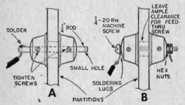
brass machine screw, washers, hexagon nuts and soldering lugs instead of the smooth rod. A 1/4-in. dia. threaded rod can be used in place of the machine screw, with a pair of hexagon nuts on both ends.—ARTHUR TRAUFFER.
