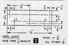
ing holes as indicated. With the strip completed, place it inside the plastic box and mark, on the plastic, the locations of the two holes marked "A". Drill  $\frac{3}{22}$  holes at these points through the plastic, and countersink them on the underside with a  $\frac{3}{22}$  twist drill.
