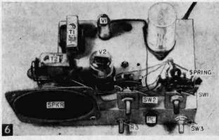
Top view of chassis of master station unit. Note spring loading (arrow) of Talk-Listen Switch.
