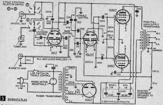
cluded here) spare lugs 4 and 5 of switch section A, and 4 and 5 of section B will accommodate these features. Note, too, that lugs 1 and 2 of switch section A are not used at any time.
