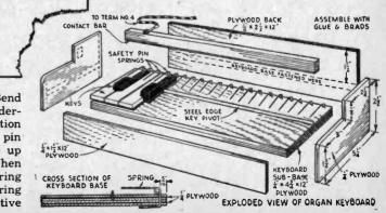
a spring through each hole. Bend projecting portion of pin on underside of base *down* (see cross-section view in plans). With all safety pin springs in place, raise each one up and slide proper key in place. When key is depressed, it will now spring back. Align and adjust each spring so that it falls in center of respective
