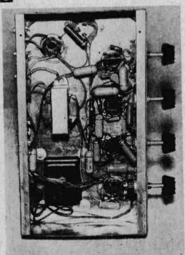
Amplifier with wiring completed.
