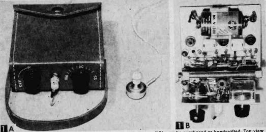
Strap allows set to be toted or tucked into pocket. Leather case (1A) may be purchased or handcrafted. Top view of simple, L-shaped chassis (1B). Loop coil snaps into fuse clips supported on spacers and a simple aluminum clip secures the miniature 9-volt transistor cell.
