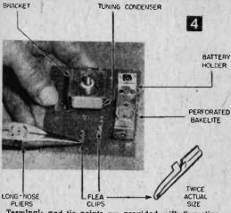
Terminals and the points are provided with flea clips that press into the holes. Use diagonal pliers to cut off the projecting ends of the clips on the other side, leaving about  $\frac{1}{22}$  in. then slightly spread the remaining ends so clips will stay in place. Insert, close-up of flea clip.
