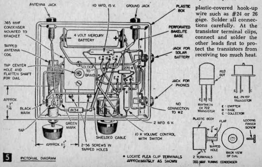
Use long-nose pliers to absorb the heat while holding each transistor lead for soldering.
