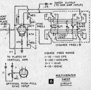
This circuitry should be well-shielded, both from the standpoint of *RF* shielding, and high-voltage protection. Usually the high-voltage supply, complete in its shielding, can be transferred from the TV set.
