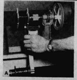
Variable speed, foot-control switch regulates speed of motor when winding coil. Photo A shows how magnet whre is hand guided from spool to coil windings.
