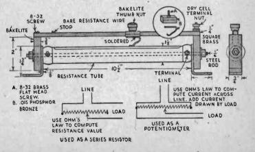
sort from a tubular adjustable resistor, or one that is equipped with an adjusting band. These can be purchased in most any radio supply store and many of them are included in surplus equipment. The advantage of a slide wire resistor is that the resistance can be adjustable in very gradual steps by simply sliding the movable unit along the wire to the point desired.
