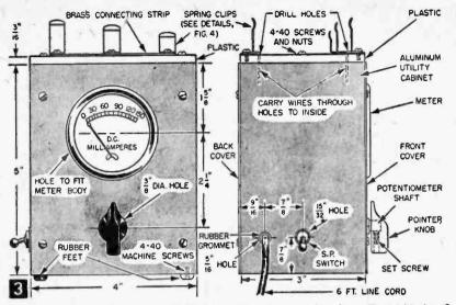
positive strip at the front. Mark the strips for quick identification. Always place cells in the clips with the positive terminals toward the front.
