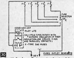
built with five fuses. By increasing the size of the switch and adding fuse Holders, even greater selection would be available. The unit is designed to use 3AG fuses; these are available in sizes from 10 ma. to 8 amps.
