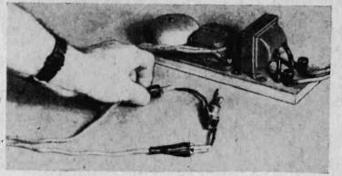
This handy door-bell and transformer unit is used for a variety of low resistance testing. In photo above it is used to find the common terminal of an S.P.D.T. switch. Drawing below shows how hookup is made.
