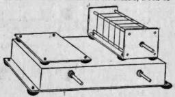
sembly panel cushioned and held to chassis, and chassis itself cushioned from operating table. In latter case, cups also keep chassis from sliding and scratching furniture. Cups are sold in most supply stores.—ARTHUR TRAUFFER.
