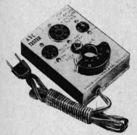
A radio and television tube filament checker such as the one shown above will test TV picture tubes as well as ordinary vacuum tubes.
