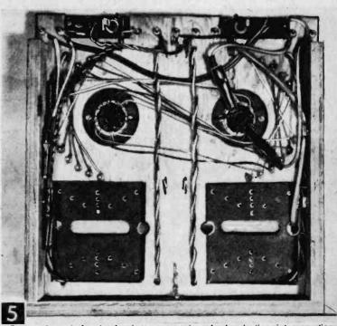
Bottom view of chassis showing permanent, underchassis tie-point connections. Note filament clips in place on right-hand tube socket.
