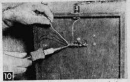
Soldering connections at terminal strip on back.
