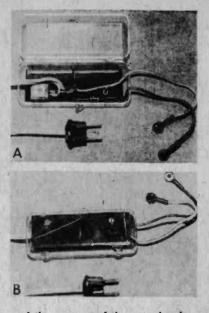
ored the reverse of the actual polarity required. Thus, black or yellow lead will be *plus*, and red lead *minus*. Snaps are wired as in Fig. 4 regardless of lead color.
