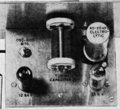
Fig. 2. Chassis provides ample room for using standard-size single-gang capacitor instead of the miniature type shown above. (With standard size, insulate rotor plates from chassis.)
