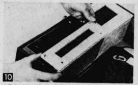
Fitting amplifier compartment back and cover in place. Below is the finished record player.
