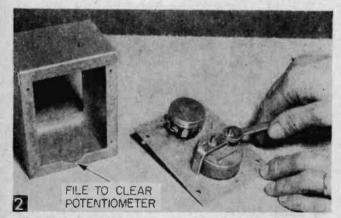
Variable resistor has been mounted to the front cover and meter is being installed. Note curve filed in case for clearance.
