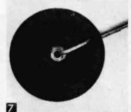
Boftom view of mike base showing how cable passes through protecting spring and up into stand tube. OD steel spring into the hole (Fig. 7). The microphone is now ready to be wired up and the can closed.
