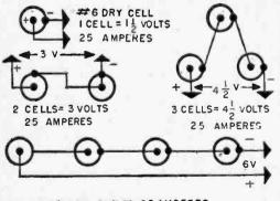
4 CELLS = 6 VOLTS 25 AMPERES SERIES CONNECTIONS OF SINGLE DRY CELLS VOLTAGE OFICELLX NUMBER OF CELLS = VOLTAGE OF GROUP. CURRENT REMAINS AMPERAGE QF 1 CELL. 2 CELLS IN PARALLEL 4 2 VOLTS-SERIES 4 2 VOLTS-SERIES 4 2 VOLTS-SERIES 4 2 VOLTS 50 AMPS 4 2 VOLTS 50 AMPS 4 2 CELLS IN PARALLEL 6 CELLS IN SERIES-PARALLEL 6 CELLS IN SERIES-PARALLEL
